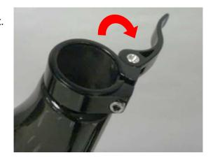
Attention: the depth of the seat post. The seat post must be inserted at least 10cm (3.9inch).
