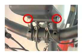
2.6.3 Adjust the angle and tighten the bracket screws.
