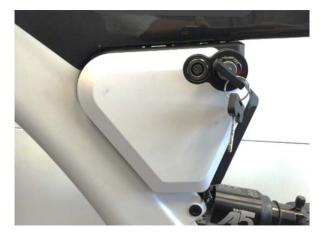
2.7.3 Push the key in and turn it to "OFF" position to lock the battery in place.
