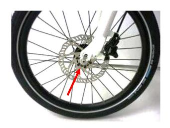
Attention: The disk should be placed between the brake pads.
